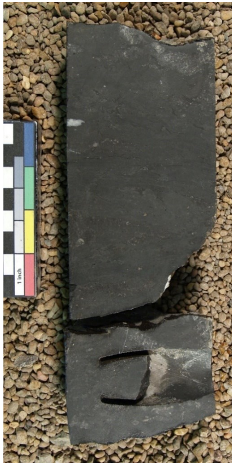
Figure 18. Alpha Marker facies core photograph. (NDIC #10480, Depth: 11,201 ft)
