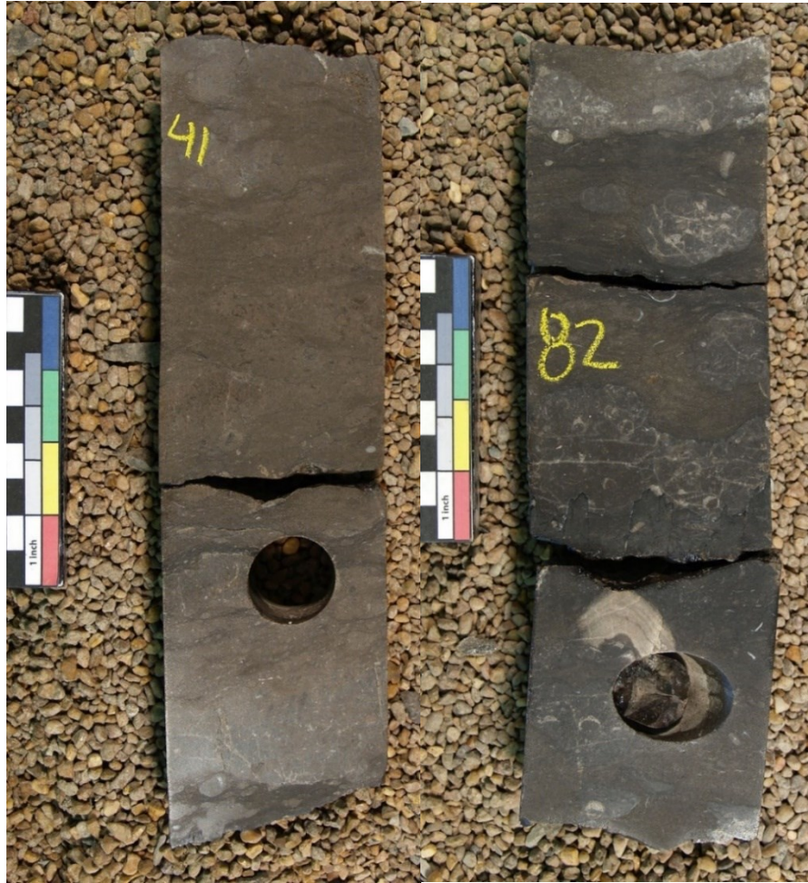
Figure 20. Brachiopod Wackestone facies core photograph. Left: (NDIC #10209, Depth: 11,141 ft). Right: (NDIC#10480, Depth: 11,182 ft)
