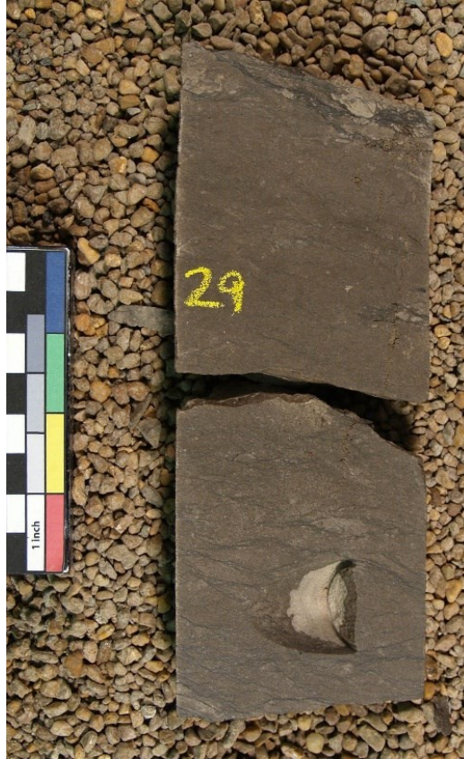
Figure 23. Dolomitic Mudstone to Wackestone facies core photograph. (NDIC #10209, Depth: 11,129 ft)
