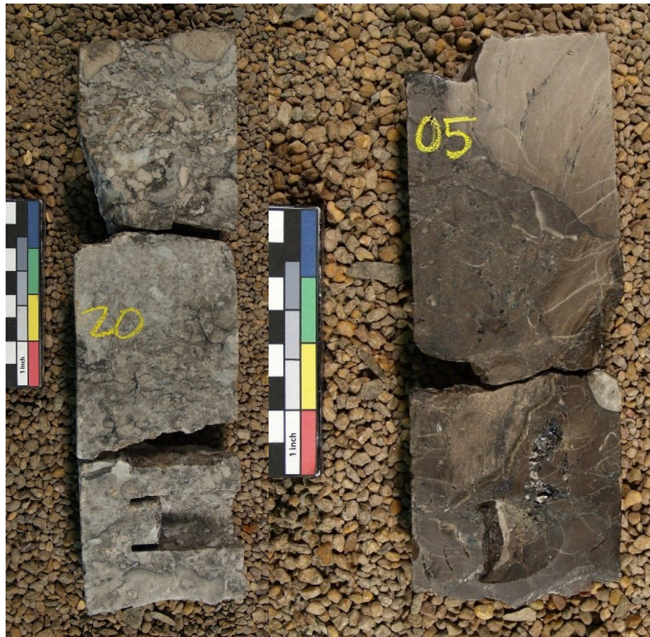
Figure 24. Reef facies core photographs. Left: (NIDC #10480, Depth 11,120 ft) Right: (NDIC #10209, Depth 11,105 ft)
